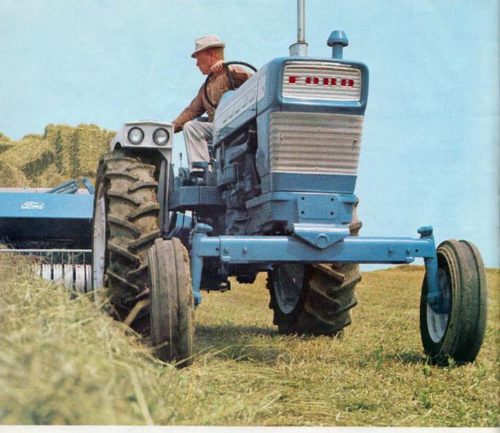
Ruggedness shows in every detail of the Ford 5000 row-crop. Optional wide front axle is built with the strength to handle heavy mounted implements—offers 2-foot under-axle clearance for row crops.
