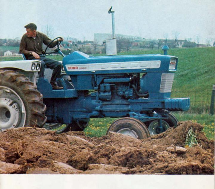
Now, get proved workpower of the Ford 5000 in a rugged row-crop model. Wide axle, shown, gives 24-inch crop clearance. Tricycle model also available. Notice the roomy operator's deck, the excellent work view. The clean design, the freedom from clutter.
