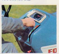
Ford's exclusive 10-speed power-shift transmission (optional) combines unsurpassed on-the-go control with efficient all-gear drive.
