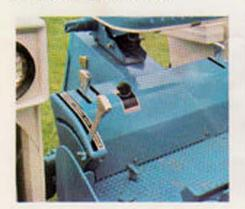
Single lever raises and lowers implements, for draft or position control. Flow control, standard. Optional remote control lever is console-mounted.
