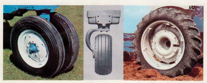
Prefer a tricycle-type tractor for use with mounted cornpickers or cultivating? Then order your 5000 with dual front wheels. Or get it with the single front wheel (center).
