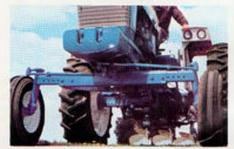
Front axle is reversible. As installed above, wheel base is 104 inches. Here, wheelbase is reduced to 88 inches. Inverted "U" channel telescopes for front tread adjustment from 56 to 88 inches.
