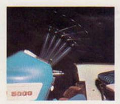
Steering wheel locks in any of 5 positions—fits you whether you sit or stand. Hydrostatic power steering takes the work out of turns.
